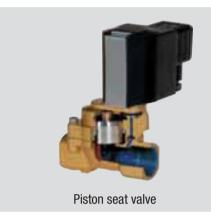
An internal piston is moved axially into the position required by the particular function. This type of valve is available in materials catering for relatively high pressure and temperature ranges.
